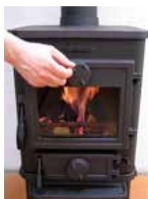
The stove door should normally be opened gently the first 2 - 3 centimetres, then you should wait until the pressure has equalised before opening the door all the way. This technique will prevent smoke from getting out, particularly when there is a poor draught.
